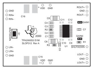
Note: Capacitors C9 – C12, C15, and C16 are optional (not assembled) and pad locations for them on the EVM PCB have been provided to increase design flexibility.
