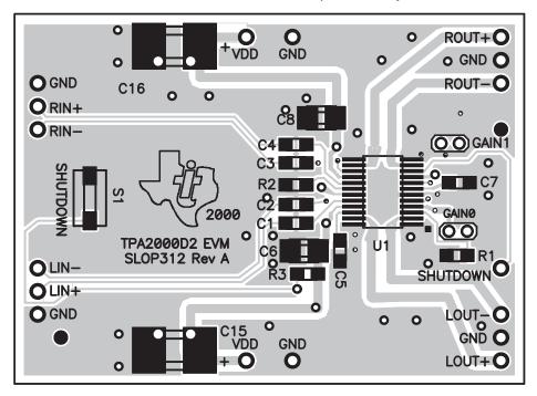
Figure 3-13. TPA2000D2 FIlterless Class-D EVM Bottom Assembly
