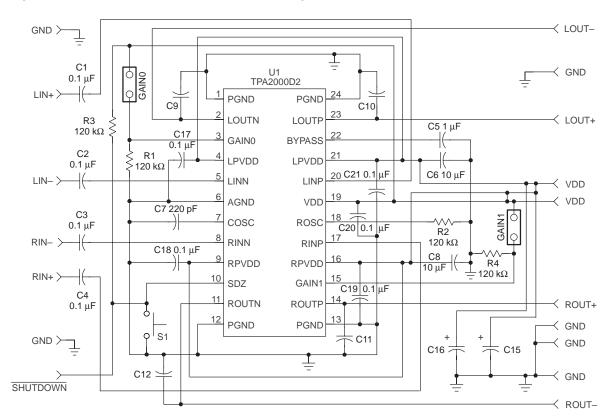
Figure 3-4. TPA2000D2 EVM Schematic Diagram
