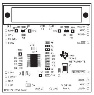
Single in-line header pins extend from the underside of the module circuit board to allow the EVM to be plugged into the TI plug-n-play audio amplifier evaluation platform, or to be wired directly into existing circuits and equipment when used stand-alone.
