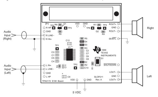
Figure 2–4. TPA0172 EVM Connected for Stereo BTL Output
