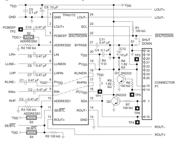
Figure 2–5. TPA0172 EVM Schematic Diagram
