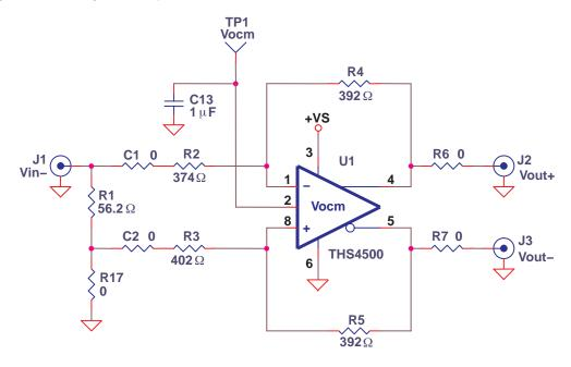
Figure 3-3. Output of an AC-Coupled, Single-Supply Application
