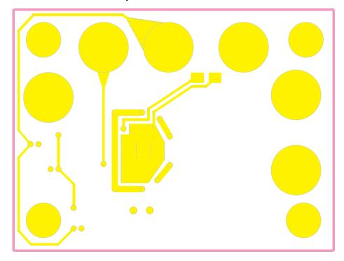
Figure 2–5. DRV593 and DRV594 Thermal Plane Layer
