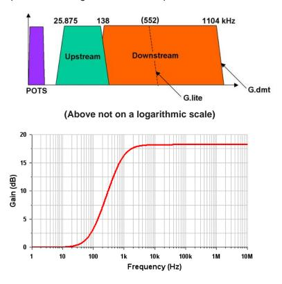
Figure 3–4. ADSL Spectrum and High-Pass Filter Response
