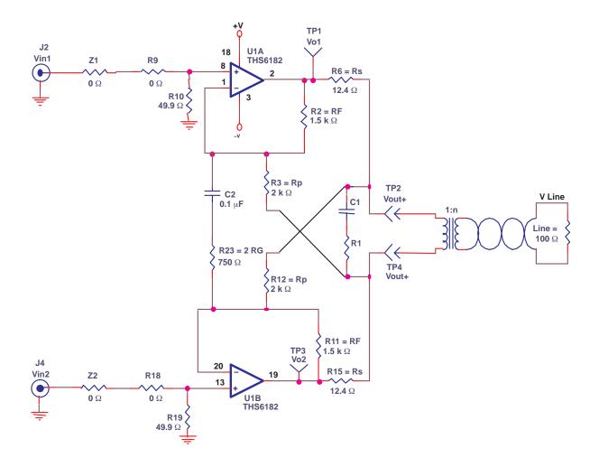
Active feedback creates larger impedance (Z) than what is actually placed there by series resistors  $R_S$ :
