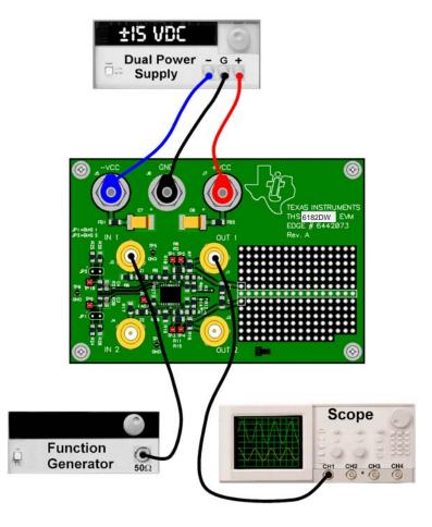
Figure 2–1 shows the connections to measure the output signal of output 1 while a single-ended signal is inserted into EVM channel 1's noninverting input. If the oscilloscope input is connected to J3 and the signal source is connected to J2, EVM channel 2 is also configured for a noninverting signal path. When the oscilloscope's input impedance is 50  $\Omega$ , the voltage gain from J2 to J3 is 1.33 V.
