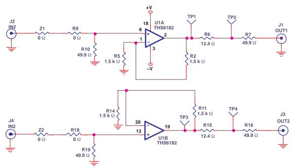
Figure 3–5. Single-Ended Amplifier Configuration
