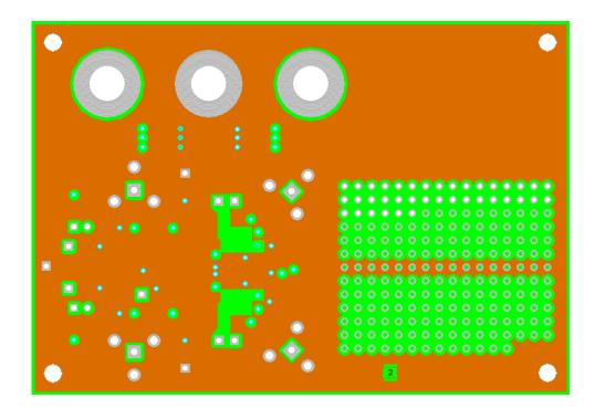
Figure 4–3. Internal Plane (Layer 3) (Power Plane)
