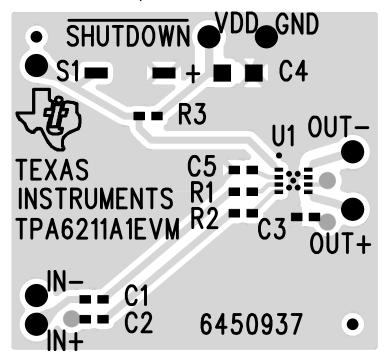
Single in-line header pins are mounted to the underside of the module circuit board. These pins allow the EVM to be plugged into the TI plug-n-play audio amplifier evaluation platform or to be wired directly into existing circuits and equipment when used stand-alone.
