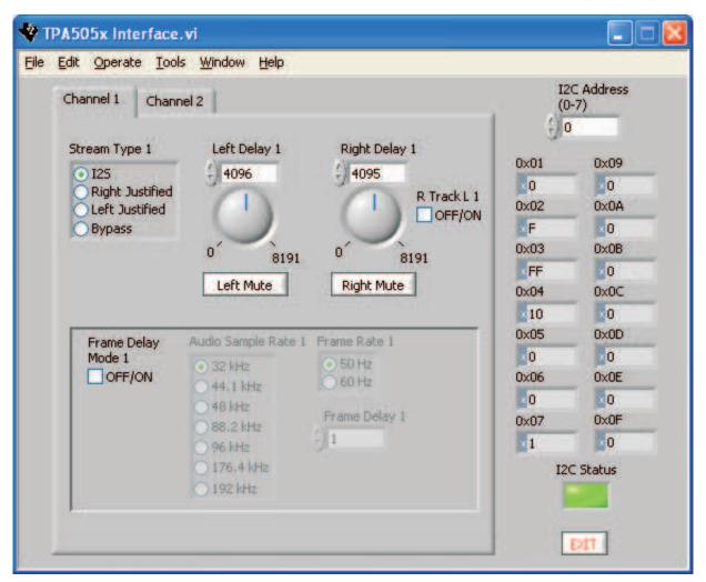
Figure 1. TPA5050 in I<sup>2</sup>S Mode With Separate Delays for Left and Right Channels
