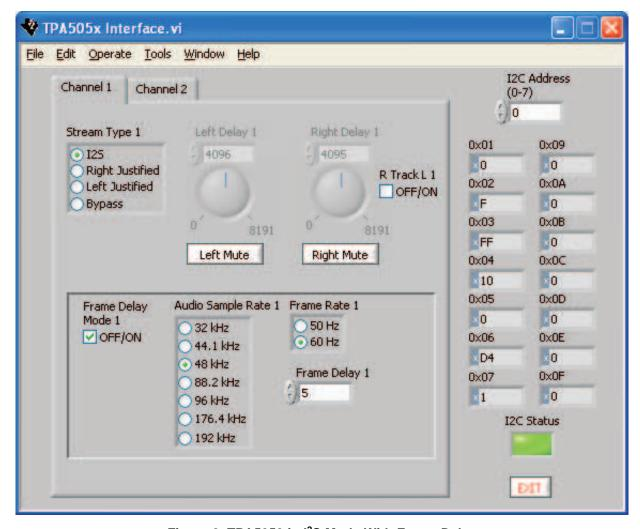
Figure 2. TPA5050 in I<sup>2</sup>S Mode With Frame Delay
