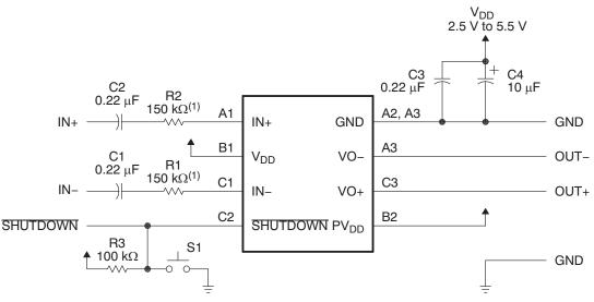
(1) Values shown are for EVM revision A only. For non-rev A EVMs, R1 = R2 =  $60.4 \text{ k}\Omega$ , A<sub>V</sub> = 5 V/V.
