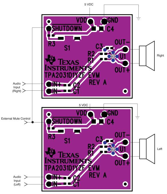
NOTE: Due to the very small size of the NanoFree<sup>™</sup> WCSP IC package, the standard part number TPA2031D1 is replaced with the code AKO (Pb-free version).
