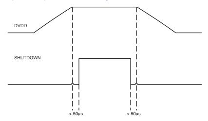
Figure 4. Power-Up/Down Sequence
