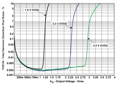
Figure 9. THD+N vs Voltage (100- $\Omega$  load) Linear Scale
