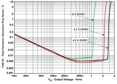
Figure 6. THD+N vs Voltage (600  $\Omega$ )
