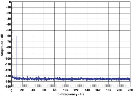
Figure 14. FFT Spectrum With –60-dBFS Tone
