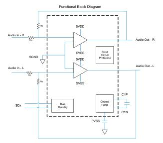
Figure 2. DRV601 Functional Block Diagram
