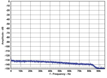
Figure 15. Idle Noise FFT Spectrum (BTL)
