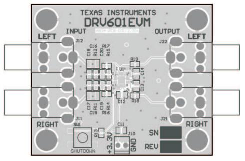
Figure 22. DRV601EVM PCB Component Placement Top
