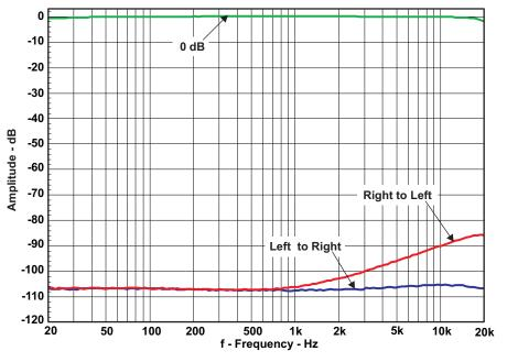
Figure 17. Channel Separation, 10x Lower Feedback Impedance
