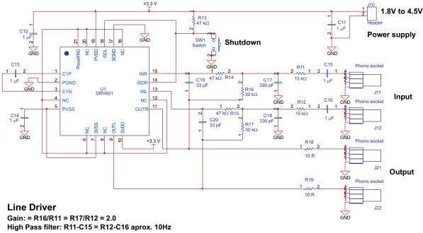
Low Pass filter: 40kHz 2nd Order Butterworth Layout note: Do not ground the powerpad - keep it floating Place C12-C13-C14 close to U10
