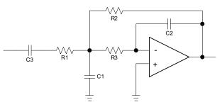
Figure 5. Second-Order, Active Low-Pass Filter
