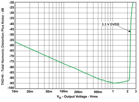
Figure 11. THD+N vs Voltage (100-kΩ Load)
