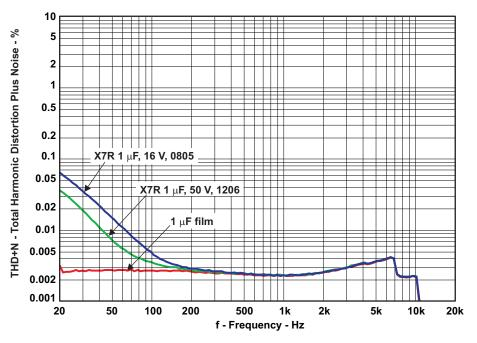
Figure 13. THD+N vs Frequency (600- $\Omega$  Load) Using X7R Input Capacitors
