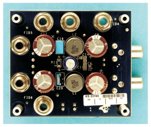
Figure 2. TPA3124D2 Audio Power Amplifier EVM – Bottom View
