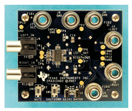
Figure 1. TPA3124D2 Audio Power Amplifier EVM - Top View
