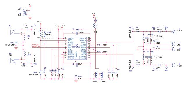
Figure 3. TPA3124D2EVM Schematic
