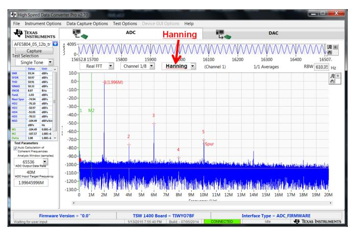
Figure 22. Analysis of Noncoherent Sampled Data
