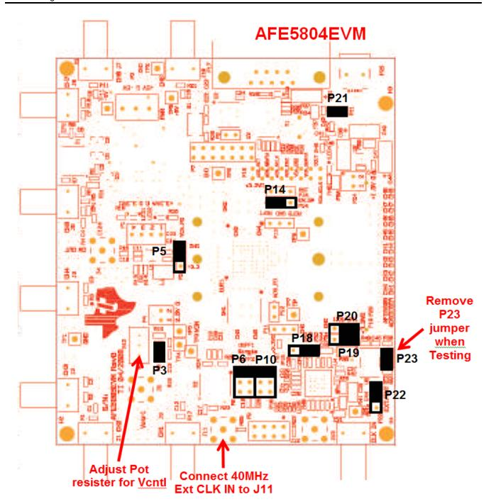
Figure 4. Default Setup for Jumpers
