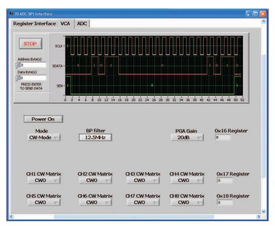
Figure 6. AFE5804EVM USB SPI Interface for CW Mode
