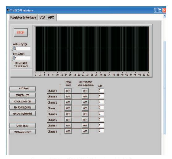
Figure 7. AFE5804EVM USB SPI Interface for ADC Setup
