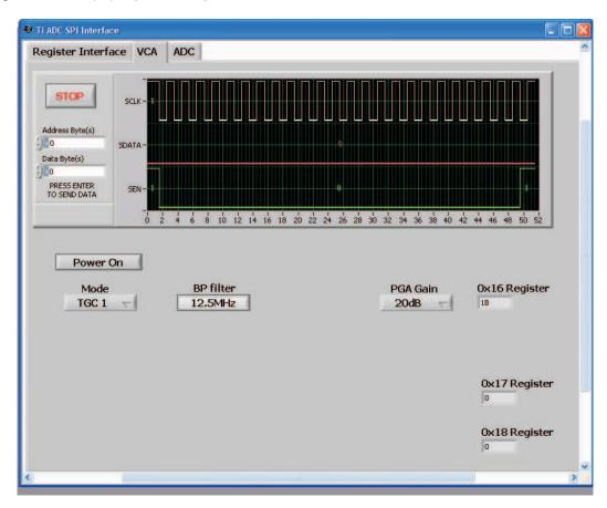
Figure 5. AFE5804EVM USB SPI Interface for TGC Mode
