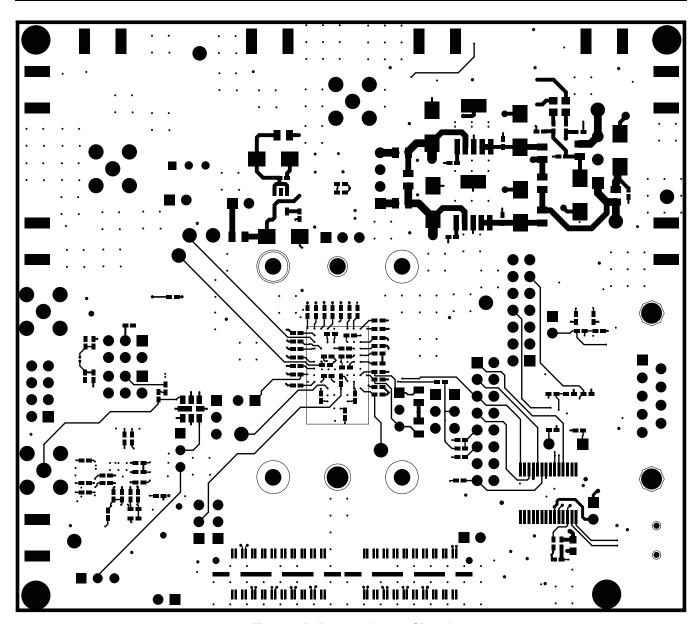
Figure 15. Bottom Layer, Signal
