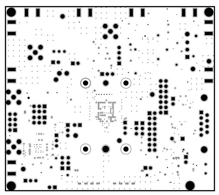
Figure 14. Inner Layer 4, Ground
