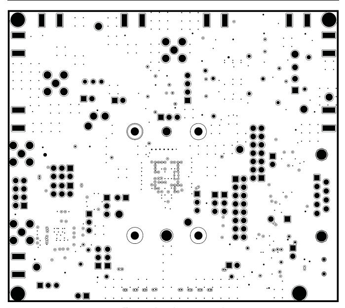
Figure 11. Inner Layer 1, Ground
