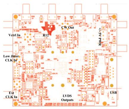
Figure 2. AFE5804EVM I/O Connectors and Locations
