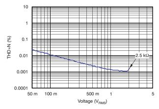
Figure 5. THD+N versus Voltage (Digital Input)
