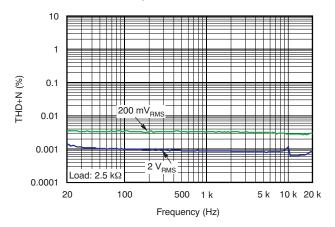
Figure 6. THD+N versus Frequency (Analog Input)
