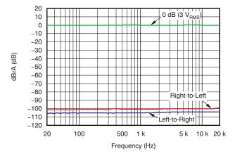
Figure 12. Channel Separation (Analog Input)
