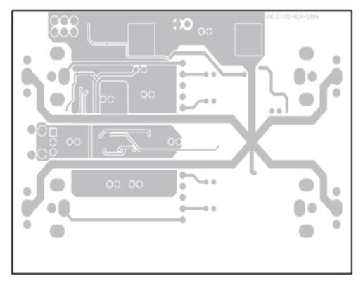
Figure 24. DRV603EVM PCB Bottom Layer
