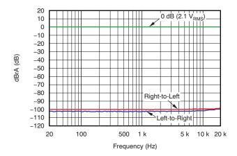
Figure 13. Channel Separation (Digital Input)
