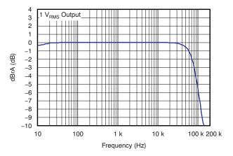
Figure 14. Frequency Response (Analog Input)
