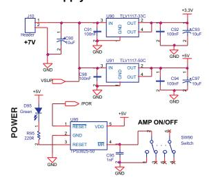
Figure 21. DRV603EVM Schematic: TOSLINK and Power Supply
