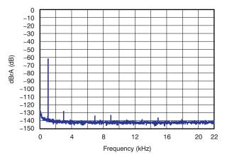
Figure 8. FFT Spectrum with -60-dBFS Tone (Analog Input)
