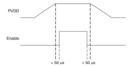
Figure 2. Power-Up/-Down Sequence
