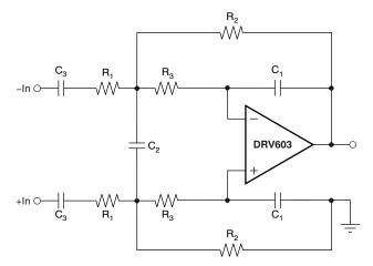
Figure 3. Differential Input, Second-Order, Active Low-Pass Filter
