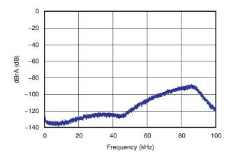
Figure 11. Idle Noise FFT Spectrum (Digital Input)
