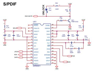
Figure 20. DRV603EVM Schematic: S/PDIF Receiver
