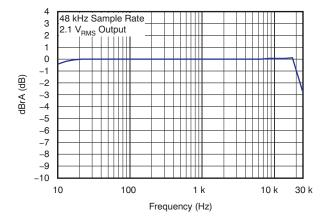
Figure 15. Frequency Response (Digital Input)
