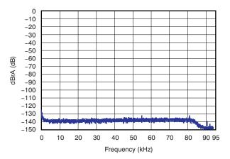
Figure 10. Idle Noise FFT Spectrum (Analog Input)
