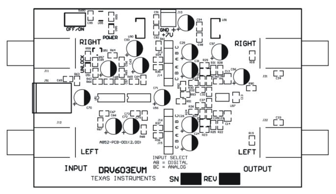
Figure 22. DRV603EVM PCB Component Placement
