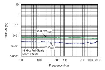
Figure 7. THD+N versus Frequency (Digital Input, 0 dBFS)
