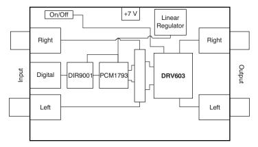
Figure 1. DRV603EVM Functional Block Diagram
