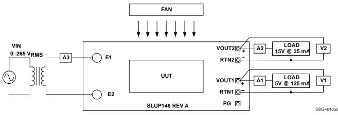
Figure 2. Dual Ouput EVM Test Configuration
