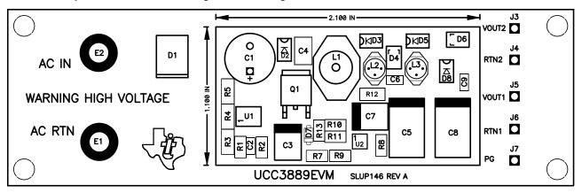
Figure 4. Top Side Component Assembly
