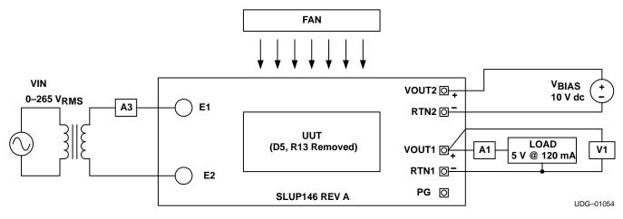
Figure 3. Single Ouput EVM Test Configuration
