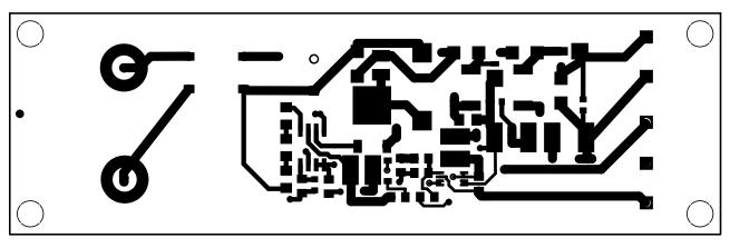
Figure 5. Layer 1 Signal Trace Layer
