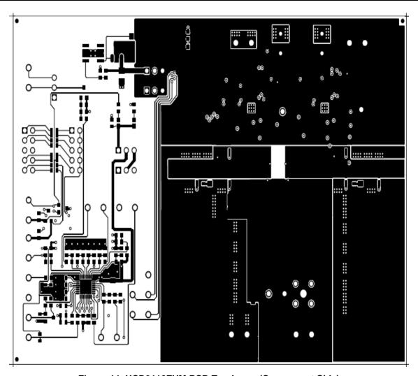
Figure 14. UCD9112EVM PCB Top Layer (Component Side)
