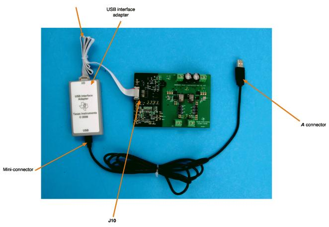
Figure 2. Connection Between EVM and Host
