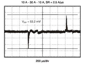
Figure 8. Output Voltage Ripple
