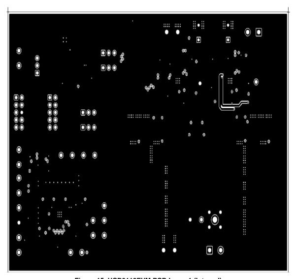
Figure 15. UCD9112EVM PCB Layer 1 (Internal)
