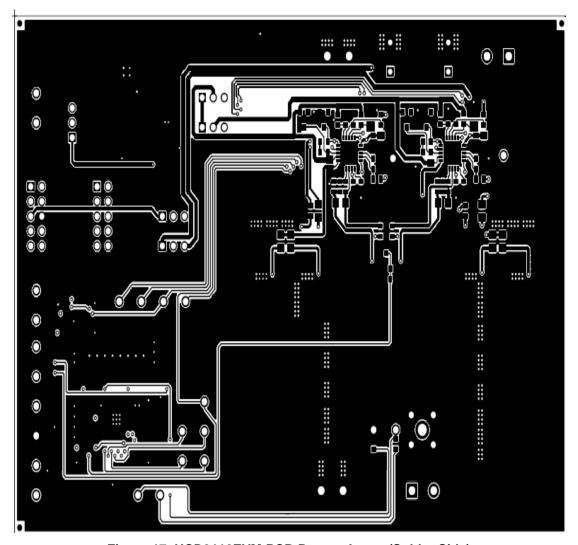
Figure 17. UCD9112EVM PCB Bottom Layer (Solder Side)
