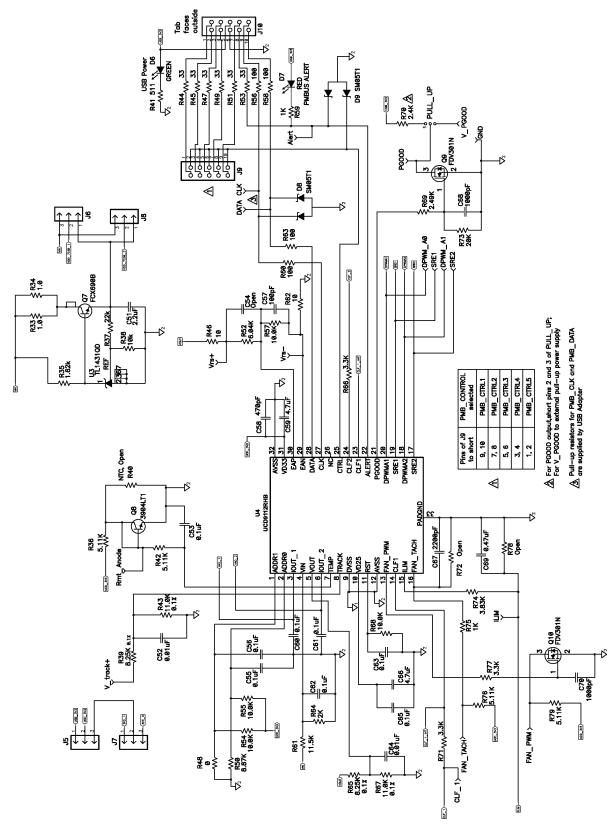
Figure 11. UCD9112EVM Schematic
