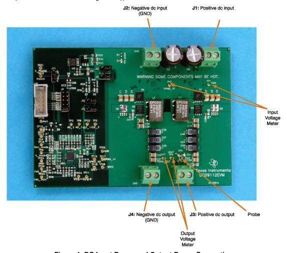
Figure 1. DC Input Power and Output Power Connection
