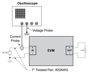
Figure 2. EVM Setup For Measuring Current-Limit
