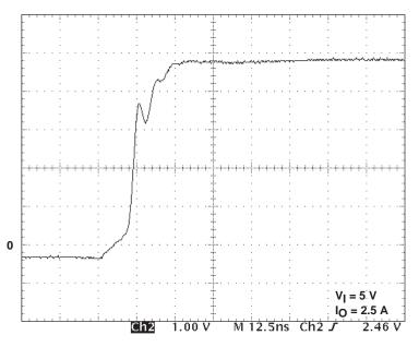
Figure 1–14. Power Switch Fall Time
