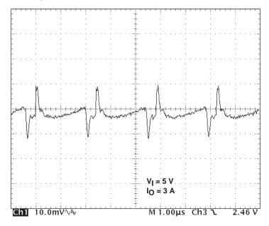
Figure 1-16. Load Transient Response
