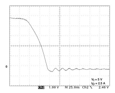
Figure 1–15. Output Voltage Ripple
