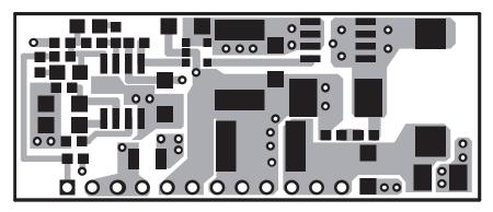
Figure 1–5. Bottom Layer (Top View)
