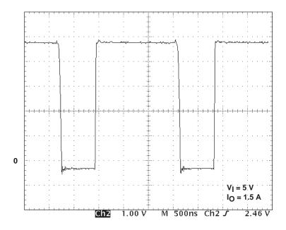
Figure 1–13. Power Switch Rise Time
