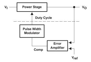
The following is a simplified approach to designing networks to stabilize continuous mode buck converters that works well when the open-loop gain is below unity at a frequency at least one-half of the switching frequency of the power supply.
