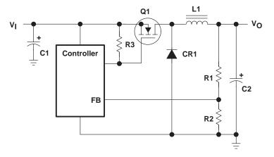
These Converter Modules are designed to provide I/O power (3.3 V) and Internal Core power (2.5 V, 1.8 V for Rev. 3 devices) to the Texas Instruments TMS320C6201 DSP. These modules satisfy all of the requirements for powering this high performance DSP such as low cost, low parts count, good transient response and excellent output voltage accuracy.
