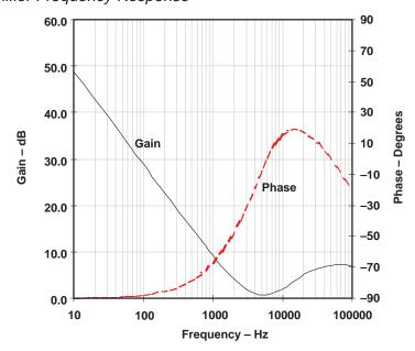
The overall open-loop frequency response of the converter is the product of the uncompensated open-loop response (Figure 2–2) and the error amplifier response (Figure 2–4). A Bode plot of the overall open loop frequency response of the converter is shown below in Figure 2–5. Again, the solid line is the gain and the dashed line is the phase. As seen in the graph, the gain crosses 0 dB in the vicinity of 20 kHz and the phase margin is approximately 100 degrees.
