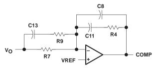
The first step in the design of the error-amplifier frequency response is the design of the output sense divider. This sets the output voltage, and the top resistor, R7, determines the relative impedance of the rest of the compensation design. A 1-k $\Omega$  resistor for the top of the divider gives a divider current of 2.3 mA for an output setting of 3.3 V and a Vref of 1 V. The bottom of the divider (omitted from Figure 2–3 for clarity) is calculated as:
