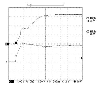
Figures 3–2 shows the same measurement as in Figure 3–1 except for a longer time period. It demonstrates the operation of the TPS70751 supervisory circuit RESET output (CH3).
