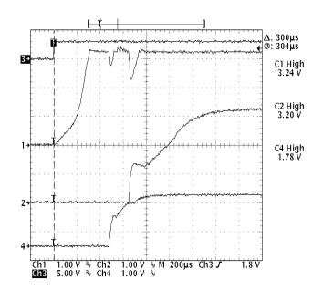
Figures 3–5 shows an ac measurement of the TPS60120, 3.3-V output, with each TPS70751 output loaded with 100 mA.
