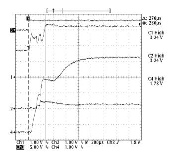
Figures 3–4 is the same as Figure 3–3 except that the TPS60120 (CH1) now has a 1 mA load and the Schottky diode between the TPS70751 has been removed. This figure shows the startup curves if no Schottky diode is used.
