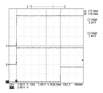
Figures 3–3 shows the startup curves of the TPS60120, 3.3-V output(CH1), and the TPS70751, 3.3-V output (CH1) and 1.8-V output (CH2). Switch SW1 was disconnected and the TPS60120 ENABLE (CH3) pin was enabled using a pulse generator. Both TPS70751 outputs have 1 mA loads. The TPS60120 output is distorted due to the load on the charge pump from the charging of the TPS70751 output capacitors and the 1 mA loads.
