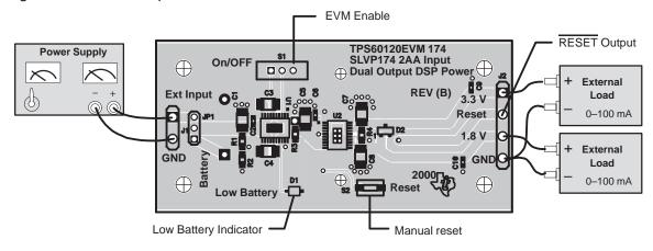
Figure 2–1. Test Setup
