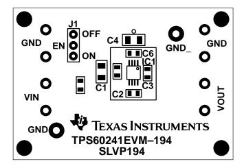
The total space required for the IC and the capacitors on the EVM is only about  $10~\text{mm}\times12~\text{mm}=120~\text{mm}^2.$  The capacitors are not optimized for space. They are optimized for performance. It is possible to use smaller capacitors to optimize the layout for minimum board space. On the EVM, it is also possible to solder some other capacitors because 1206-size pads have ben added in parallel to  $C_{IN}$  and  $C_{OUT}$ .
