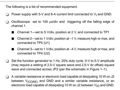
The following steps are recommended for evaluating the power-up sequencing of the two devices:
