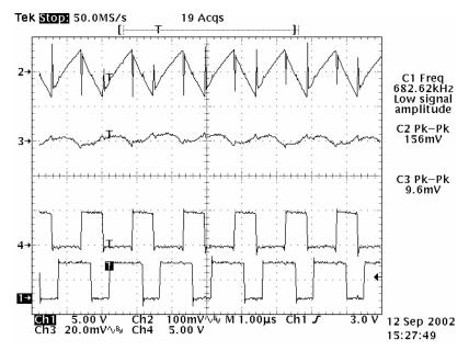
Figure 2-17. Input and Output Voltage Ripple and Main Switching Waveform at  $V_I = 5 V$
