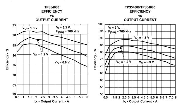
The input current, consumed by 3.3-V output regulator TPS54x10, is excluded from these data. The measurements relate only to the core voltage channel provided by tracking regulators TPS54680 and TPS54880. Efficiency is lower at higher ambient temperatures, due to temperature variation in the drain-to-source resistance of the MOSFETs. The efficiency is slightly lower at 700 kHz than at lower switching frequencies, due to the switching losses in the MOSFETs.
