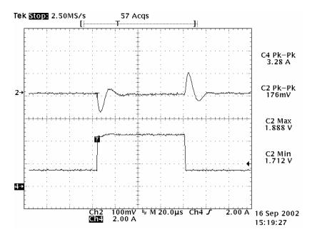
Figure 2-13. Load Transient Response at Input Voltage 5 V, TPS54680/TPS54880
