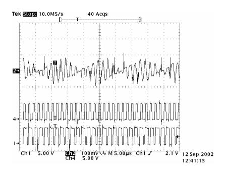
Figure A-2. Input Voltage Ripple (Ch.2),Sync Signal (Ch.3) and Switching Waveforms of Core Regulator (Ch.4) and I/O Regulator (Ch.1)
