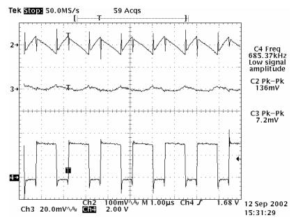
Figure 2-17 shows the output and input voltage ripple and main switching waveforms of the core regulator TPS54680/TPS54880 and I/O regulator TPS54610/TPS54810. The measurements are taken at V<sub>I</sub> = 5 V, V<sub>O</sub> = 1.8 V (core), I<sub>O</sub> = 6 A (core), V<sub>O</sub> = 3.3 V (I/O), I<sub>O</sub> = 0 A (I/O) and Fs = 700 kHz for both channels. For these waveforms:
