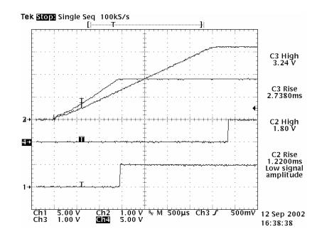
Figure 2-6. Powering Up With Core Voltage Rising FIrst
