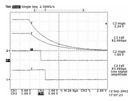
If jumper JP2 is set so that R2 is connected in parallel to R3, the core voltage rises first during power up, i.e. prior to the I/O voltage rise, and falls second during power down. The waveforms with this type of sequencing are shown in Figure 2-6 and Figure 2-7.
