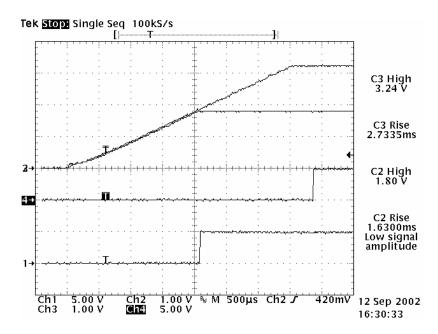
The powering down waveform, by using the ENABLE signal, is shown in Figure 2-3. During power down, the fall time of output voltage depends on the output capacitance and load resistance. In this case a very low resistance (0.5  $\Omega$ ) I/O output load has been selected to show the dynamic performance of the TPS54x80. It is seen that even if the I/O output voltage falls with the slew
