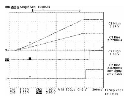
Figure 2-5. Powering Down With Ratiometric Sequencing
