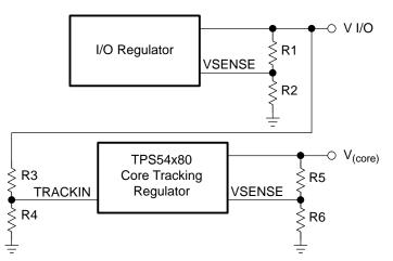
Implementation of different power sequencing techniques is based on proper resistor-divider ratio selection. The equations 1, 2, and 3 provide related ratios for different ways of power sequencing.
