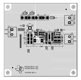
Figure 3–6. Bottom Side Assembly (Showing Optional Components)
