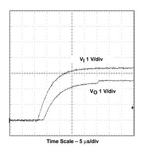
Figure 2–20, Figure 2–21, and Figure 2–22 show the same series start-up waveforms for the TPS54873-225. The above descriptions of the TPS54673 waveforms are applicable for the TPS54873 except that the input voltage is 5 V, the output voltage is 3.3 V, and the UVLO start-up threshold is 3.8 V.
