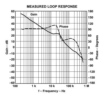
Figure 2–12. Measured Loop Response, TPS54873, V<sub>I</sub> = 6 V
