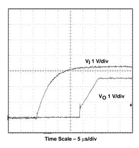
Figure 2–18 Shows the start-up waveform with the output precharged and a 2- $\Omega$  load. The precharge is achieved by connecting the 3.3-V input to the output with two diodes in series. The start-up mechanism is the same as described above except that the internal reference must ramp up above the voltage fed back from the precharged output to the VSENSE pin before switching can start. Once this occurs, the output continues to ramp up to the output set point of 2.5 V at the slow-start rate.
