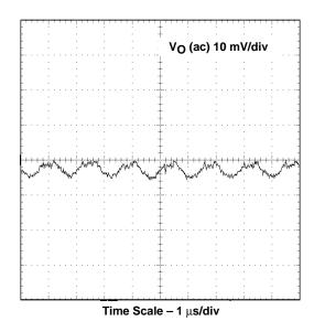
Figure 2–14. Measured Output Ripple Voltage, TPS54873
