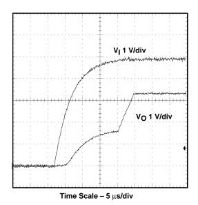
Figure 2–22. Measured Start-Up Waveform, TPS54873 With Precharge and No Load
