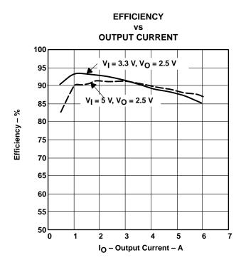
Figure 2–3. Measured Efficiency, TPS54873
