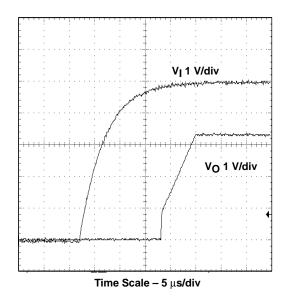
Figure 2-21. Measured Start-Up Waveform, TPS54873 With Precharge
