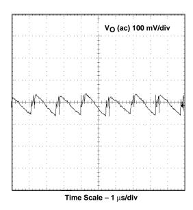
Figure 2-16. Input Voltage Ripple, TPS54873
