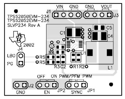
Figure 3-2. Component Placement
