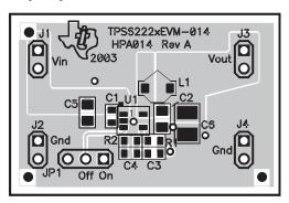
Figure 3-2. Top Layer Routing
