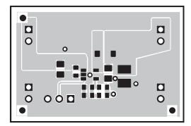
Figure 3-3. Bottom Layer Routing
