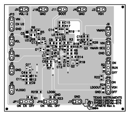
Figure 3–2. Top Layer Routing
