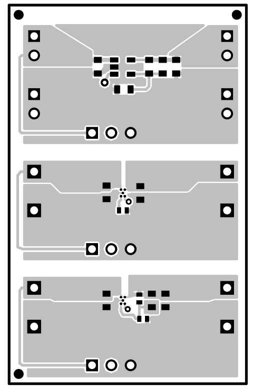
Figure 2. Top Layer Routing
