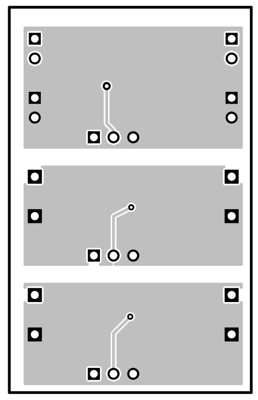
Figure 3. Bottom Layer Routing
