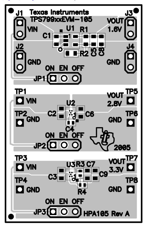
Figure 1. Assembly Layer
