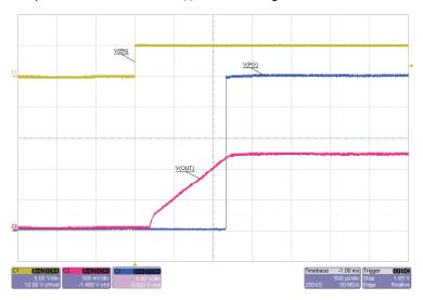
$V_{IN}$  = 1.8 V,  $V_{BIAS}$  = 5.0 V,  $I_{OUT}$  = 500 mA
