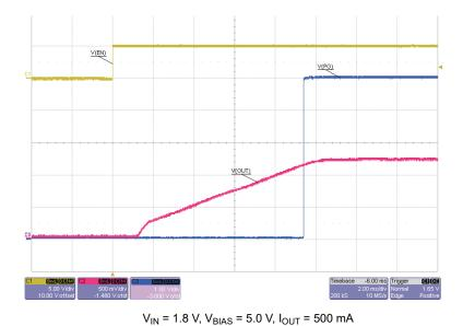
Figure 4-2. TPS74701 and TPS74801 Start-Up in 10 ms With PG
