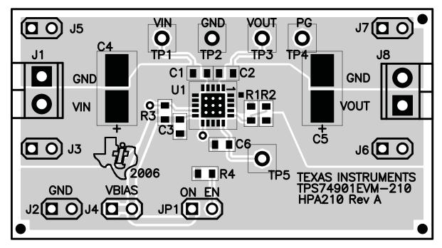
Figure 2. Top Assembly Layer
