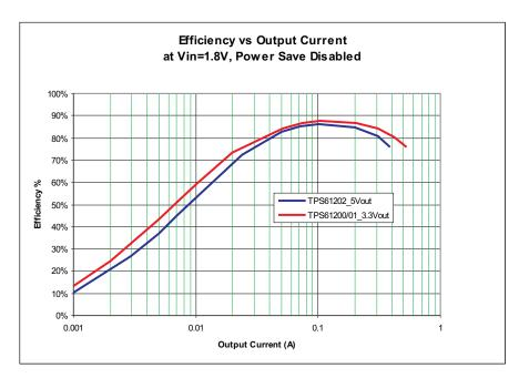
Figure 2. Efficiency vs Output Current
