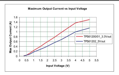
Figure 1. Maximum Output Current vs VBAT
