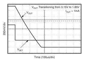
Figure 2. VSET Toggled High to Low,  $I_{OUT} = 1 \text{ mA}$
