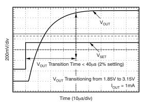
Figure 1. VSET Toggled Low to High,  $I_{OUT} = 1 \text{ mA}$
