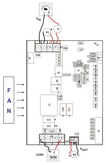
Figure 3. TPS40180EVM Recommended Test Set-Up
