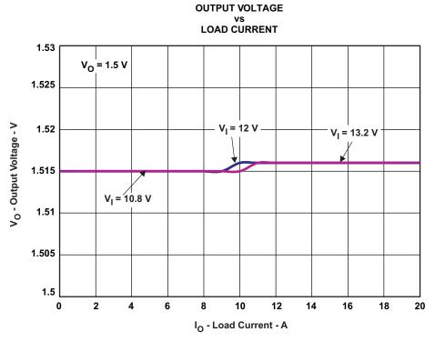
Figure 7. TPS40180EVM V<sub>OUT</sub> = 1.5V Load Regulation
