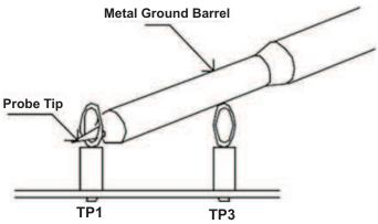
Tip and Barrel Output Ripple Measurement
