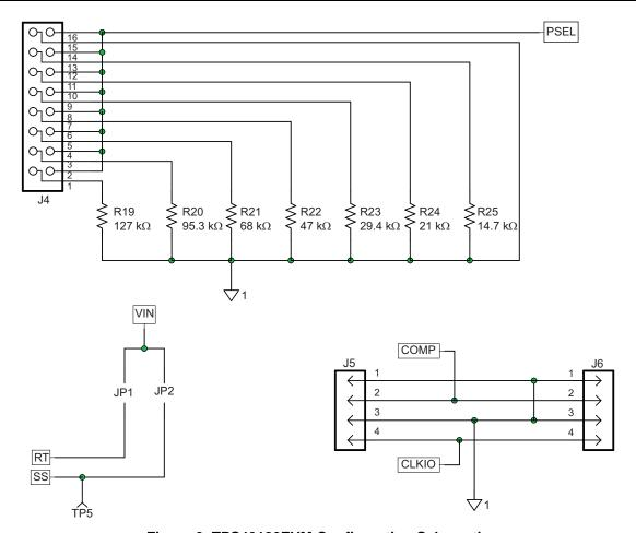
Figure 2. TPS40180EVM Configuration Schematic
