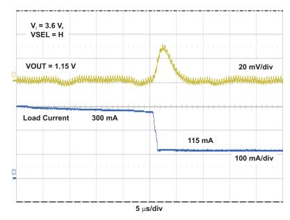
Figure 3. Load Transient, 300 mA to 115 mA step,  $V_I$  = 3.6 V, VOUT = 1.15 V
