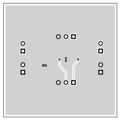
Figure 10. Bottom Layer Routing
