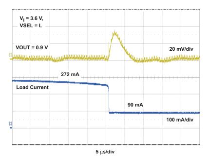
Figure 6. Load Transient, 272 mA to 90 mA step,  $V_1 = 3.6$  V, VOUT = 0.9 V
