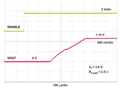
Figure 1. Start up from Enable, VI = 3.6 V, VOUT = 1.15 V, R<sub>Load</sub>= 2.5  $\Omega$
