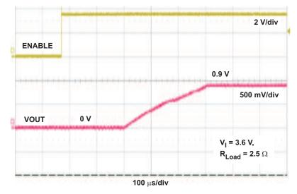
Figure 4. Start up from Enable, V<sub>I</sub> = 3.6 V, VOUT = 0.9 V, R<sub>Load</sub> = 2.5  $\Omega$
