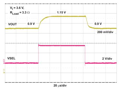
Figure 7. VSEL Output Voltage Response, V<sub>I</sub> = 3.6 V, R<sub>Load</sub> = 3.3  $\Omega$
