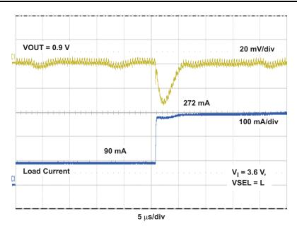
Figure 5. Load Transient, 90 mA to 272 mA step,  $V_1$  = 3.6 V, VOUT = 0.9 V
