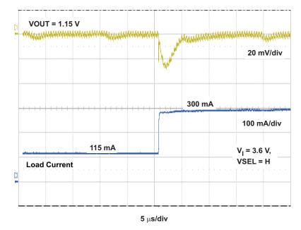
Figure 2. Load Transient, 115 mA to 300 mA step,  $V_1 = 3.6$  V, VOUT = 1.15 V
