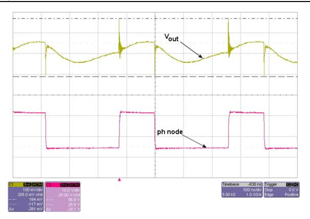
Figure 5. Measured Output Voltage Ripple, TPS5430
