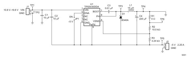
Figure 10. TPS5430EVM-342 Schematic
