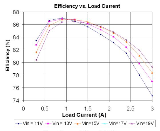
Figure 1. Measured Efficiency, TPS5430
