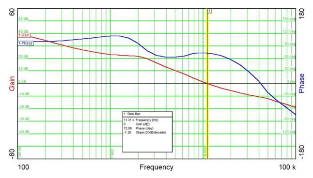
Figure 4. Measured Loop Response, TPS5430, V<sub>IN</sub> = 12 V
