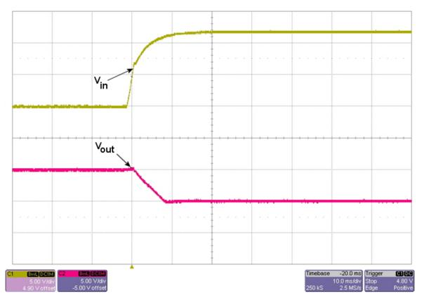
Figure 6. Power Up, V<sub>OUT</sub> Relative to V<sub>IN</sub>
