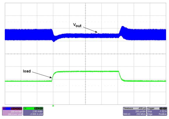
Figure 3. Load Transient Response, TPS5430
