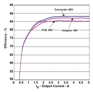
Figure 3. TPS23754EVM-420 Efficiency With 5V Output
