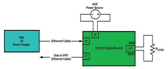
Figure 2. Typical TPS23754EVM-420 Test Setup
