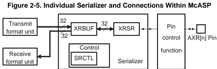
For receive, data is shifted in through the AXR[n] pin to the shift register XRSR. Once the entire slot of data is collected in the XRSR, the data is copied to the data buffer XRBUF. The data is now ready to be read by the DSP through the RBUF register, which is an alias of the XRBUF for receive. When the DSP reads from the RBUF, the McASP passes the data from RBUF through the receive format unit and returns the formatted data to the DSP.
