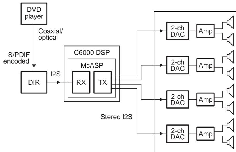
**Figure 1-2. McASP to 6-Channel DAC and 2-Channel DAC**
