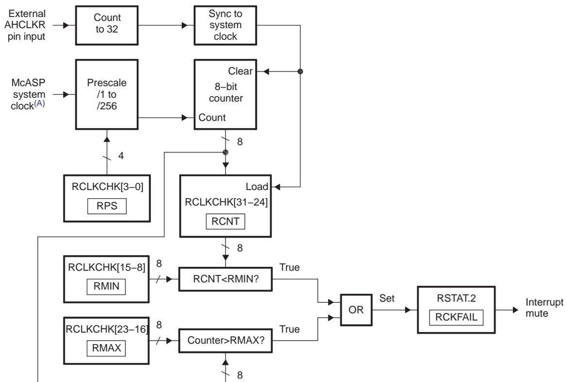
A Refer to device data manual for the McASP system clock source. This is not the same as AUXCLK.
