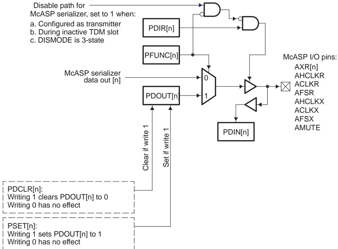
**Figure 2-9. McASP I/O Pin to Control Register Mapping**
