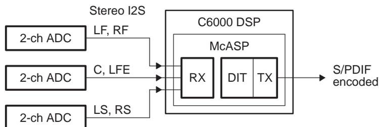
**Figure 1-5. McASP as 16 Channel Digital Processor**
