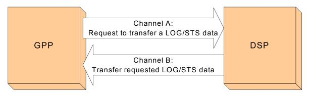
Figure 1-2. Typical RTA SDK Data Exchange Transaction
