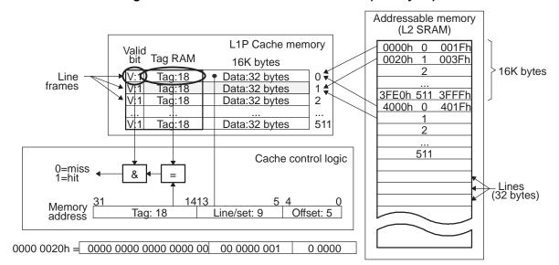
Figure 1-4. C64x+ L1P Cache Architecture (16K Bytes)
