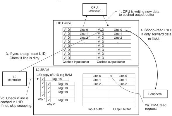
Figure 2-4. DMA Read of L2 SRAM
