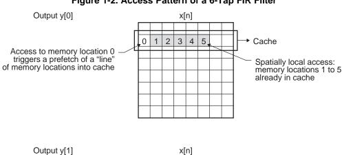
Figure 1-2. Access Pattern of a 6-Tap FIR Filter
