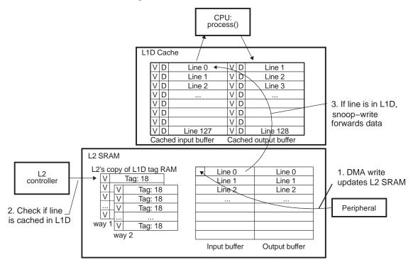
Figure 2-3. DMA Write to L2 SRAM
