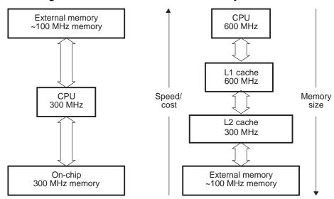
Figure 1-1. Flat Versus Hierarchical Memory Architecture
