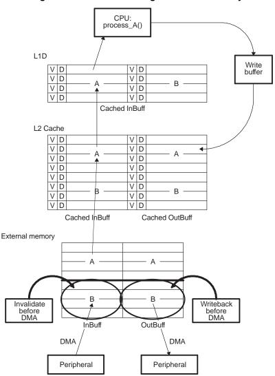
Figure 2-6. Double Buffering in External Memory
