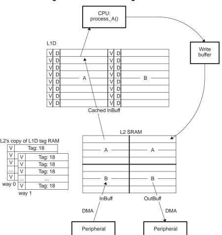
Figure 2-5. Double Buffering in L2 SRAM
