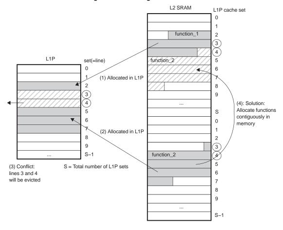
**Note:** With code generation tools 5.0 (CCS 3.0) and later, the GROUP directive **must** be used to force a specific link order.
