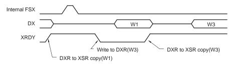
(c) XMCM = 2h, XPABLK = 0, XCERE0 = 0000 000Ah: All channels enabled, only 1 and 3 unmasked
