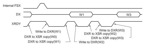
(d) XMCM = 3h, RPABLK = 0, XPABLK = x, RCERE0 = 0000 0008h, XCERE0 = 0000 000Ah: Receive channels: 1 and 3 enabled; transmit channels: 1 and 3 enabled, but only 3 unmasked
