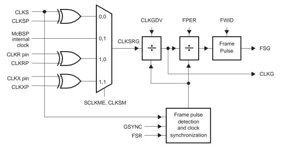
Figure 5. Sample Rate Generator Block Diagram
