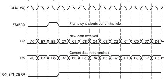
Figure 19. Unexpected Frame Synchronization With (R/X)FIG = 0
