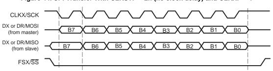
Figure 44. SPI Transfer With CLKSTP = 2h (no clock delay) and CLKXP = 1
