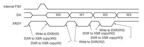
(b) XMCM = 1h, XPABLK = 0, XCERE0 = 0000 000Ah: Only channels 1 and 3 enabled and unmasked
