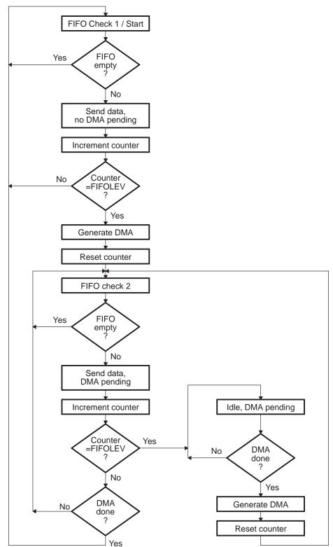
Figure 11. FIFO Operation During Card Write Diagram
