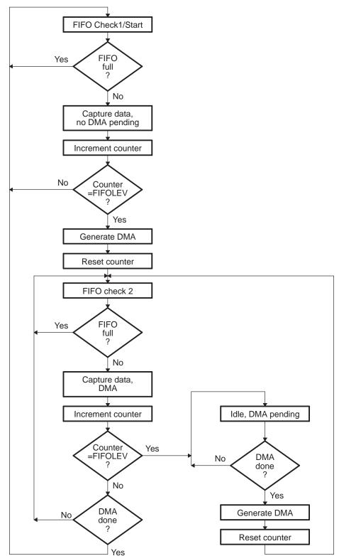
Figure 10. FIFO Operation During Card Read Diagram
