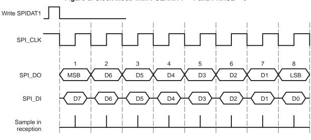
Figure 6. Clock Mode with POLARITY = 1 and PHASE = 0
