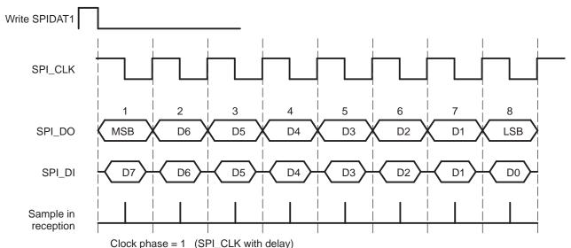
Figure 7. Clock Mode with POLARITY = 1 and PHASE = 1
