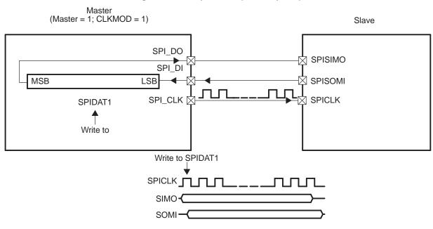
Figure 9. SPI Operation (3-Pin Option)
