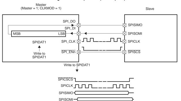
Figure 10. SPI Operation (4-Pin Option)
