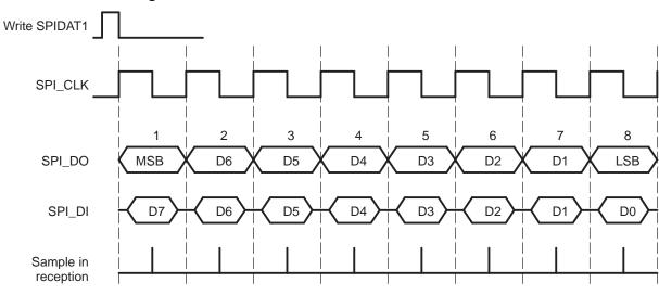
Figure 4. Clock Mode with POLARITY = 0 and PHASE = 0
