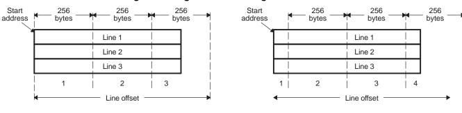
Figure 49. Alignment of Starting Address Pointer
