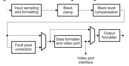
Figure 23. CCD Controller Processing Block Diagram - YUV Modes
