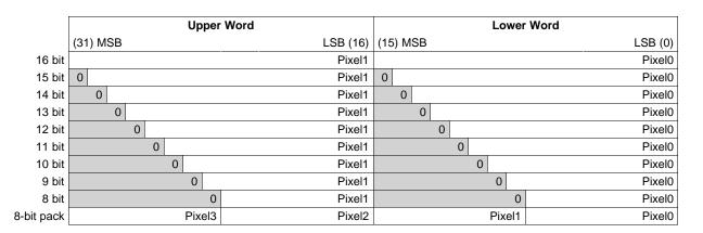
Figure 4. DDR2 Output Format
