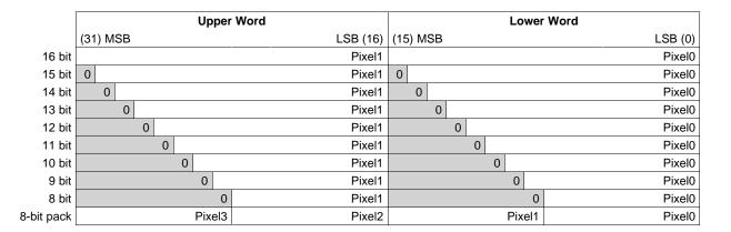
Figure 22. DDR2 Output Format
