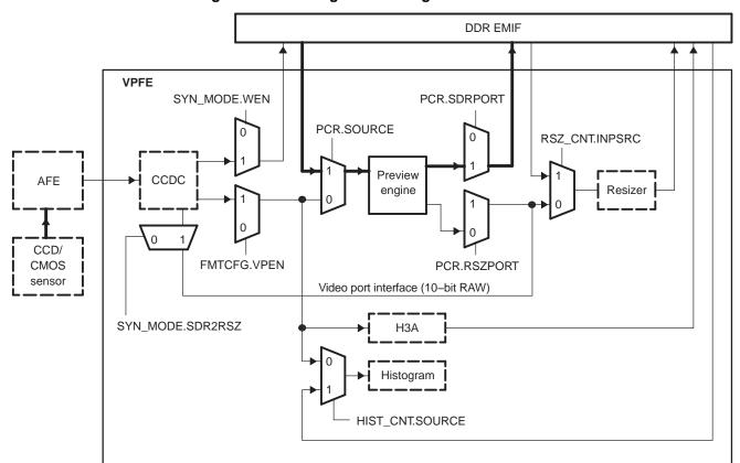
Figure 64. Still Image Processing Mode Data Path
