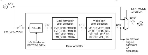
The Video Port/Data Formatter output can also be saved to DDR2 instead of the RAW CCD data. The setting SYN\_MODE.VP2SDR sends the Video Port data to the CCDC's Output Formatter. In addition, the normal DDR2 write enable (SYN\_MODE.WEN) also must be enabled to store the output to DDR2.
