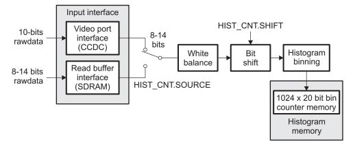
Figure 44. Histogram Processing Flow
