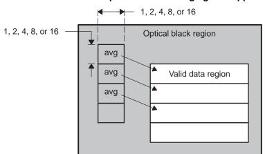
Figure 13. CCD Controller Optical Black Averaging and Application
