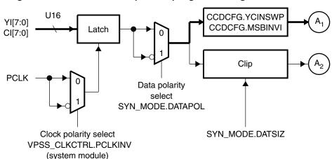
Figure 24. CCD Controller Input Sampling Block Diagram - YUV Modes
