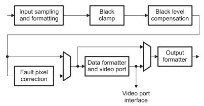
The following sections describes the CCD controller processing for the CCD/CMOS Raw Data input mode (SYN\_MODE.INPMODE = 0 && REC656IF.REC656ON = 0) in more detail. In this mode, raw sensor data, typically one color per pixel in a color filter array (or CFA) at 8 to 6 bits in dynamic range is input (usually between 10-14 bits). The color filter array applied is typically a Bayer pattern as show in Figure 10 for RGB color space.
