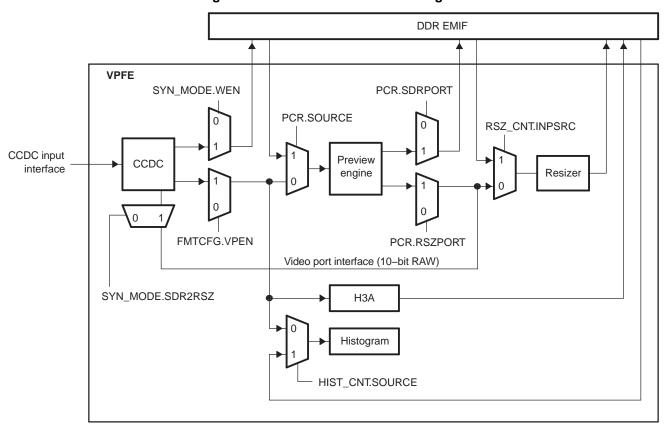
Figure 52. VPFE Data Flow Block Diagram
