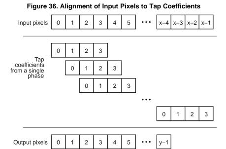
Figure 36 also presents how the first output is computed when all of the taps have been aligned with actual input pixels. In order to compute the last several pixels in each line/column, the filter needs more input pixels than the following equation calculates:
