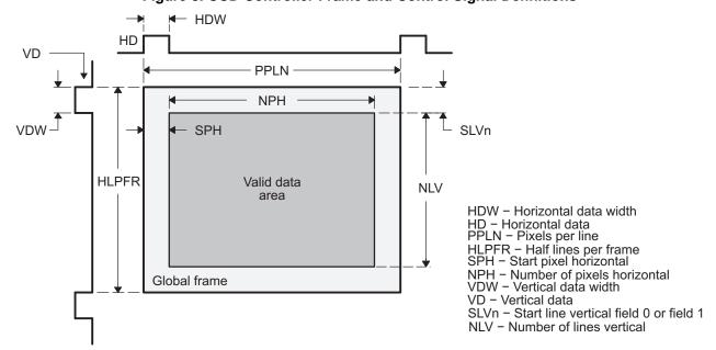
Figure 8. CCD Controller Frame and Control Signal Definitions
