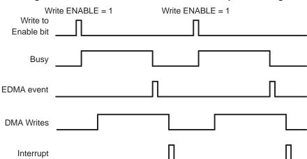
Figure 59. Firmware Interaction for SDRAM-Input Resizing
