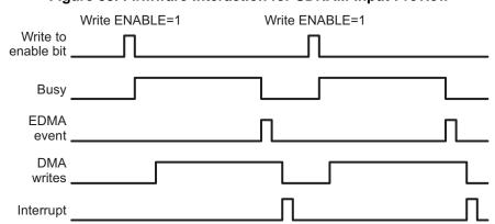
Figure 58. Firmware Interaction for SDRAM-Input Preview
