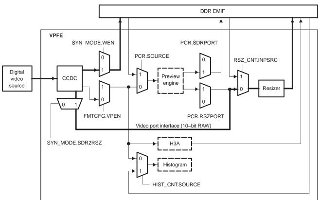
Figure 67. Video Capture Mode Data Path
