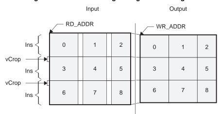
Figure 66. Horizontal Slicing Through Preview Engine
