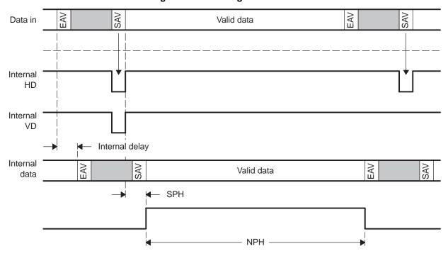
Figure 5. BT.656 Signal Interface
