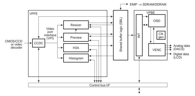
Figure 1. Video Processing Subsystem (VPSS) Block Diagram
