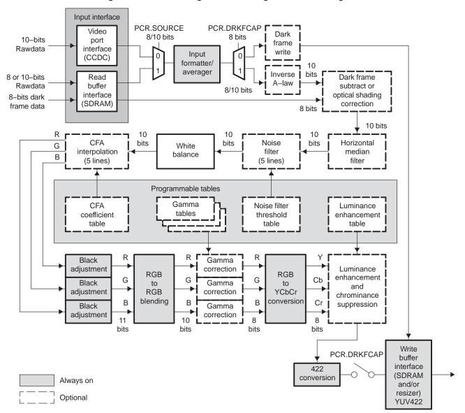
Figure 28. Preview Engine Processing Flow Block Diagram
