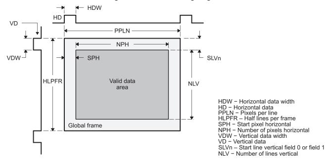
Figure 3. Raw Mode Timing Diagram
