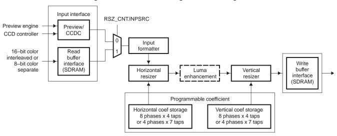
Figure 32. Resizer Processing Flow Block Diagram
