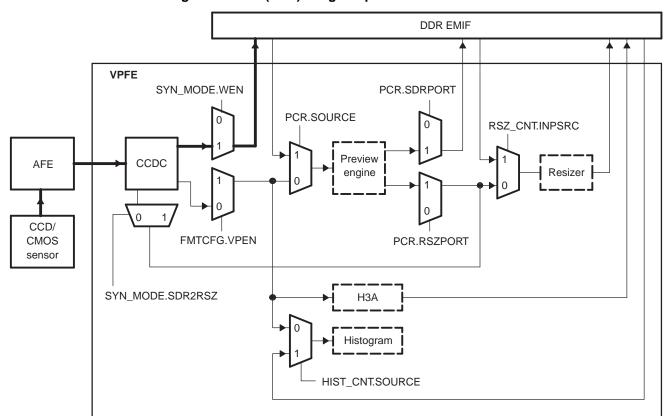
Figure 63. Still (Raw) Image Capture Mode Data Path
