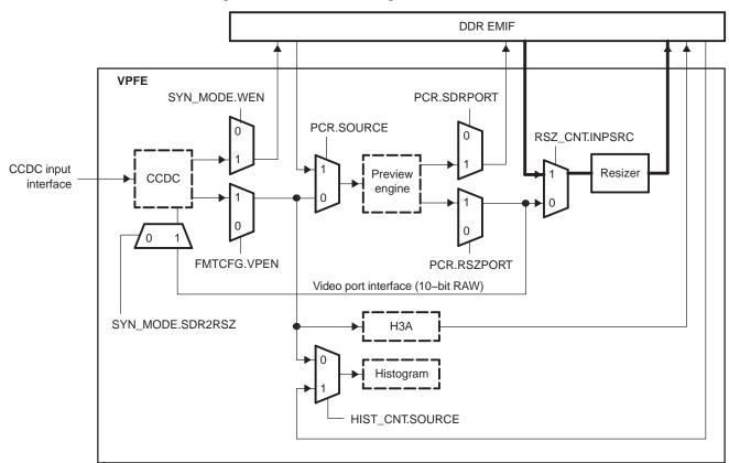
Figure 68. Processed Image Resize Data Path
