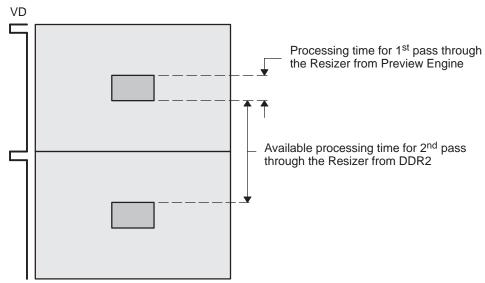
The pseudo-code in Example 4 shows the control sequence that needs to be performed by an interrupt service routine or EDMA transfer of register writes to the resizer after the resizer is initialized for the first resize. Since both passes perform up-sampling, the filter coefficients do not need to be changed once they are initially set. This example performs a 10x resize where the first pass is 4x and the second pass is 2.5x.
