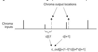
In Figure 43, the f variable represents a real-number quantity, so we use f and 1 - f for the weights in the interpolation. On the algorithm above, fixed-point arithmetic is used. The variable f is an unsigned integer representing the fraction f. Thus 1 - f becomes 512 - f is an unsigned representing 0.5 real-number, is added to the sum, then the sum is right-shifted by 9 bits to get back to the integer chroma representation.
