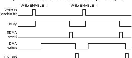
Figure 60. Firmware Interaction for SDRAM-Input Histogram
