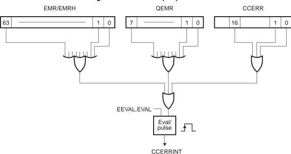
Figure 14. Error Interrupt Operation
