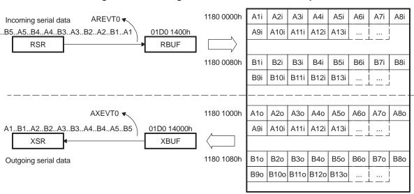
Figure 26. Servicing Continuous ASP Data Example
