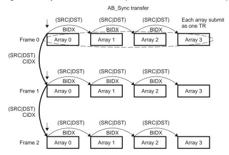
Figure 6. AB-Synchronized Transfers (ACNT = n, BCNT = 4, CCNT = 3)
