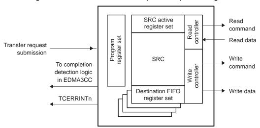
Figure 3. EDMA3 Transfer Controller (EDMA3TC) Block Diagram
