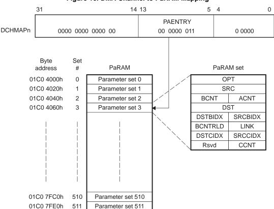
Figure 10. DMA Channel to PaRAM Mapping
