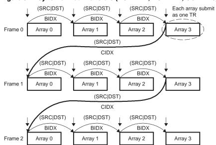
Figure 5. A-Synchronized Transfers (ACNT = n, BCNT = 4, CCNT = 3)
