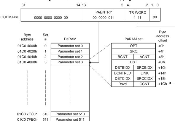
Figure 11. QDMA Channel to PaRAM Mapping
