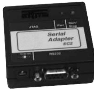
**Figure 2: EC2 serial adapter**
