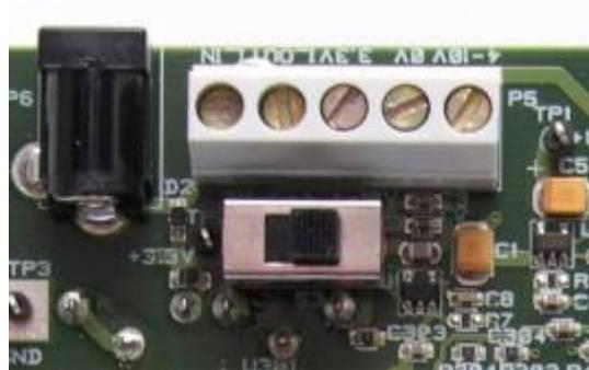
Figure 4: Power switch setting
