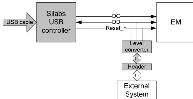
Figure 14: SmartRF<sup>®</sup>04EB used as ICE
