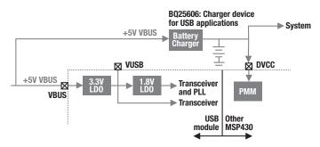
**Figure 4.** Power over USB can also be used as a primary source to charge batteries. TI's BQ2560x and BQ2407x charger families have been specifically designed for USB battery charging applications.
