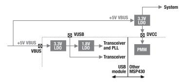
**Figure 3.** For high-current systems or for applications where it makes sense to power a device from battery even when connected via USB, the MSP430 offers the flexibility of bypassing the integrated 3.3V LDO and driving DVcc from an external supply.
