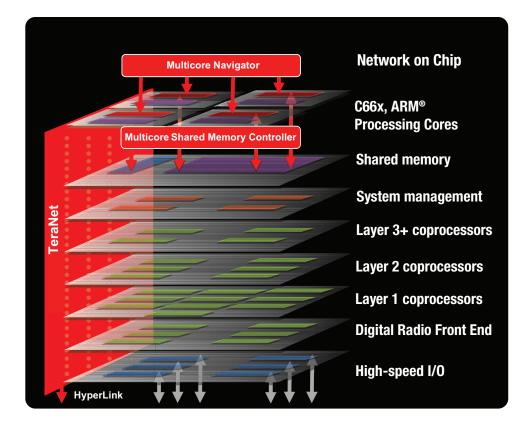
Figure 2. TI's multicore SoC architecture.
