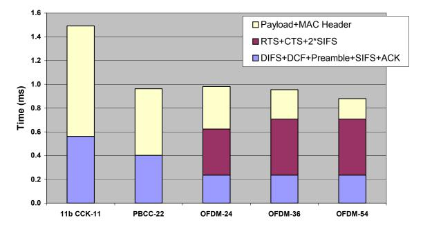
Chart 2: Time to transmit 1,000-Byte blocks using a short preamble
