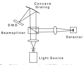
Figure 12. Schematic representation of a DMD-based digital spectrometer.
