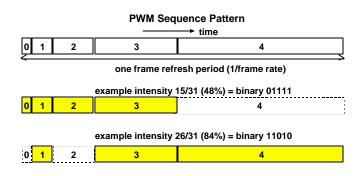
**Figure 4**. Binary PWM sequence pattern with two examples of how intensity values are generated for 5-bit video
