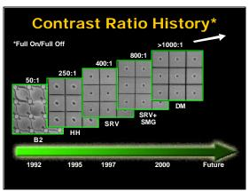
**Figure 14**. Continuous improvement in full-on/full-off contrast ratio.
