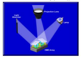
**Figure 2**. Two mirror-pixels. One mirror-pixel is turned "on" and reflects incoming light through a projection lens to the screen. One mirror-pixel turned "off" reflecting the light away from the lens.
