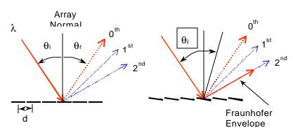
**Figure 10**. Incident light hitting a grating (DMD) with periodicity d with mirrors in flat state (on left) versus mirrors in +1 state (on right). In the "blazed" grating condition (on right), most of the diffracted radiation is concentrated in the  $2^{nd}$  order, producing a highly efficient coherent light modulator.
