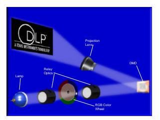
**Figure 3.** A one-chip DLP<sup>TM</sup> projection system. White light is focused down onto a spinning color wheel filter system. The wheel spins illuminating the DMD sequentially with red, green, and blue light. At the same time RGB video signal is being sent to the DMD mirror-pixels. The mirrors are turned on depending on how much of each color is needed. The eye integrates the sequential images and a full color image is seen.
