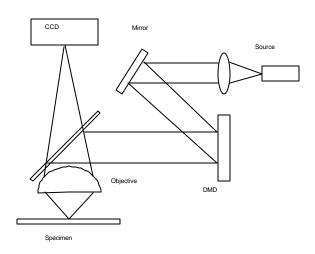
**Figure 11**. Schematic representation of an optical microscope using the DMD as a scanning aperture
