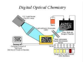
**Figure 8**. Custom biotech chip fabrication using a UVcapable DMD to pattern DNA sequences.
