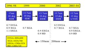
Figure 13. DMD technology advances and device formats.
