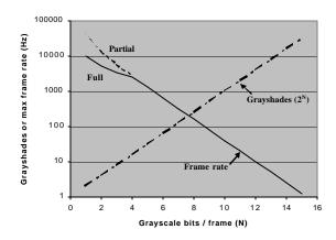
**Figure 5**. Maximum frame rate as a function of digital bits and resulting intensity levels (grayshades) possible within one frame time for the 0.7 XGA DDR DMD using the Discovery 1000 digital controller.
