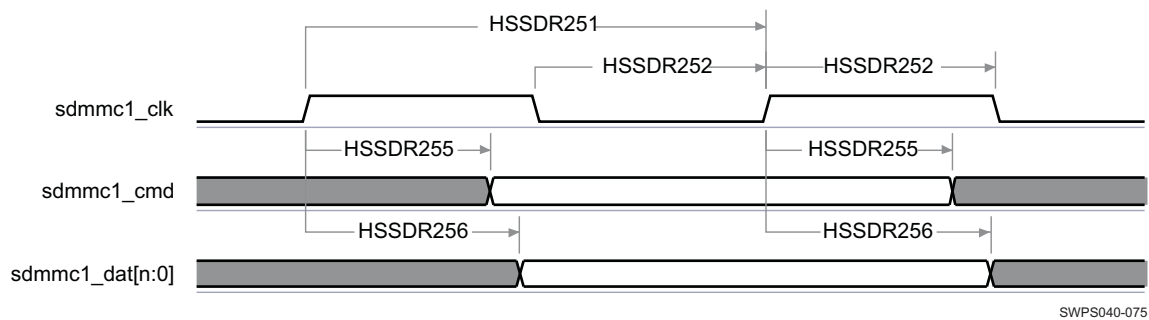
Figure 6-112. MMC/SD/SDIO 1 Interface—High-Speed SD Mode—Transmitter Mode (1)
