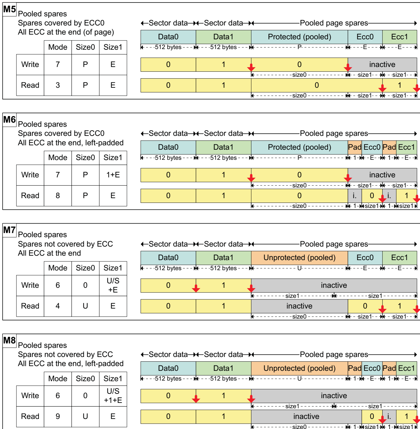
Figure 11-34. NAND Page Mapping and ECC: Pooled Spare Schemes
