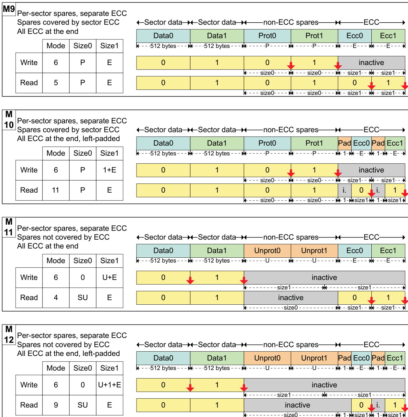
Figure 11-35. NAND Page Mapping and ECC: Per-Sector Schemes, With Separate ECC
