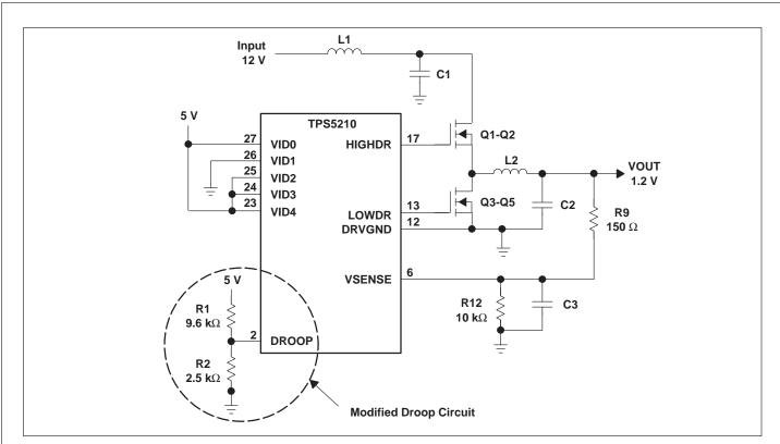
Figure 1. TPS5210 Application Circuit for 1.2-V Output
