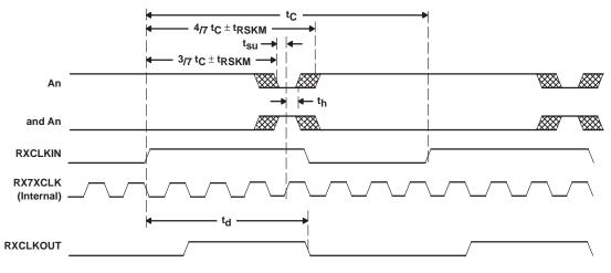
Figure 4. t<sub>RSKM</sub>, t<sub>su</sub>, and t<sub>h</sub> Waveforms
